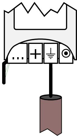
The measuring probes of this device are of the [DS18B20](#) type, its power is 3.3V and communicate with the equipment through a single cable, in the image you can see one of the probes that we supplied with the device.
